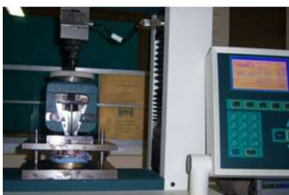
Fig.4: Impression made on universal testing machine
