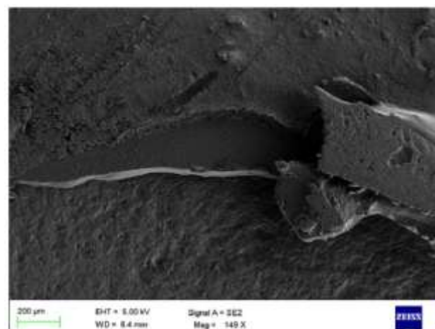
Fig. 2: SEM micrograph of a cohesive resin fracture with Fusion Self Lute™ – Prevest DenPro®
