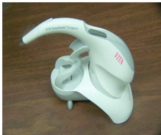
Fig. 2: Vita easy shade compact dental spectrophotometer
