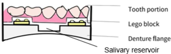
Figure 3: Designing of mandibular salivary reservoir
