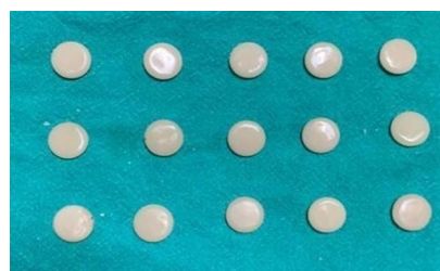
Figure 5: Polished IPS E.max CAD specimens (group 1)
