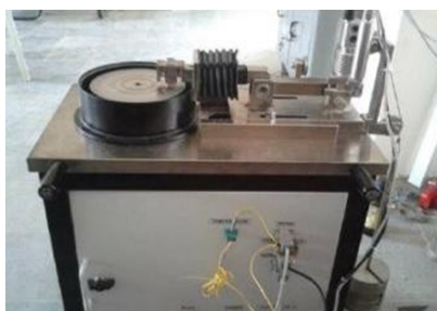
Figure 7: Pinon disc wear test machine
