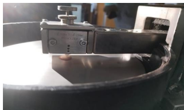
Figure 8: Enamel pin against IPS Emax CAD disc specimens.
