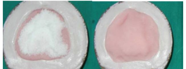
Fig. 9: Lost salt technique
