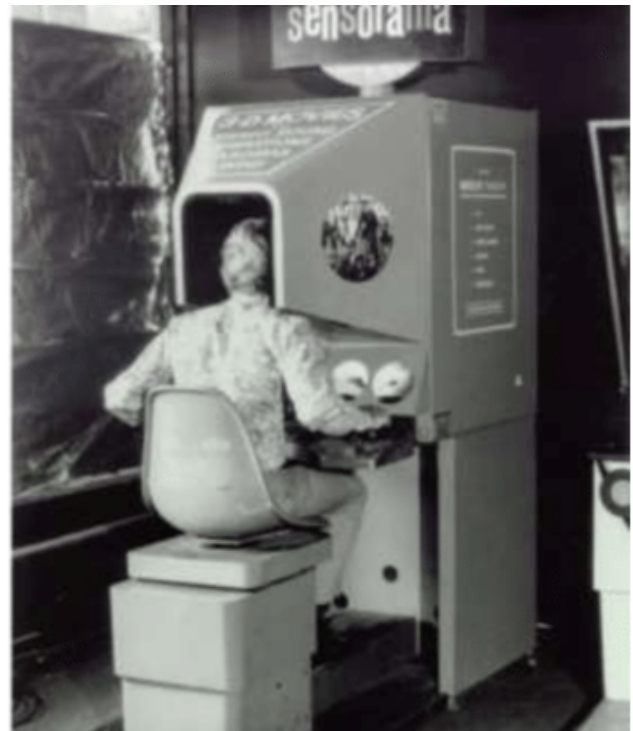
Fig. 1: SENSORAMA Sensorama Simulator patented by M. L. Heilig (1962). This invention is widely credited as being the first simulator designed to stimulate multiple senses. [Figure reproduced from Heilig (1962, Figure 5),
