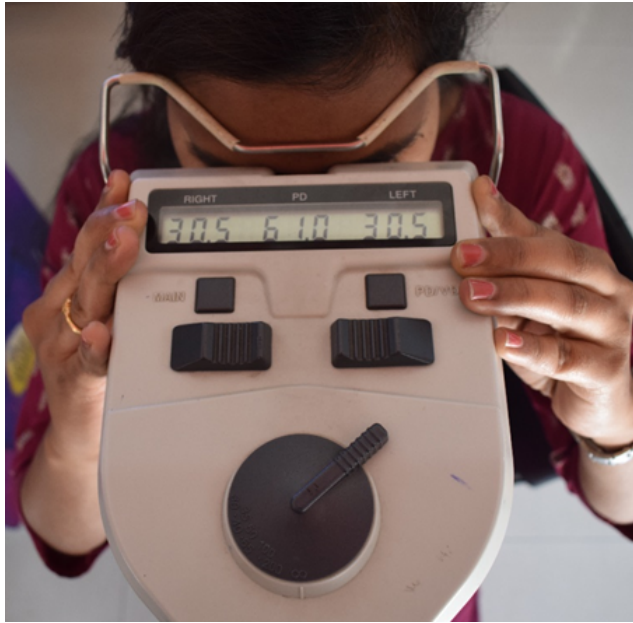
Fig. 7: Pupil Distance Meter for verification of iris position and gaze
