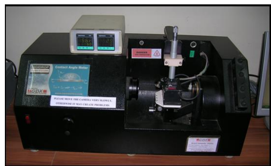
Fig. 2: Contact angle analyzer (Digidrop, Contact angle meter, GBX products, France)
