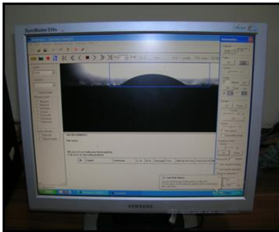
Fig. 4: Contact angle being analyzed and measured
