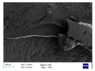
**Fig. 2:** SEM micrograph of a cohesive resin fracture with Fusion Self Lute  $^{TM}$  – Prevest DenPro®
