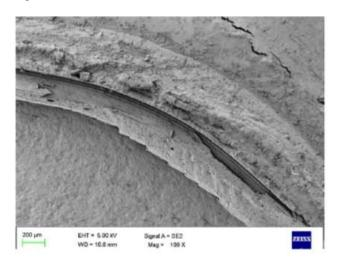
**Fig. 1:** SEM micrograph of a cohesive resin fracture with RelyX  $^{TM}$  Ultimate Clicker $^{TM}$  - 3M ESPE
