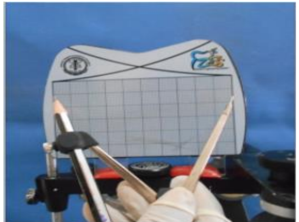
Fig. 6: Four inch radius is set for the caliper
