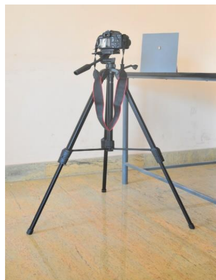
Fig. 3: Digital SLR camera placed on the tripod to obtain image of the tooth sample placed on the 18% reflectance grey card
