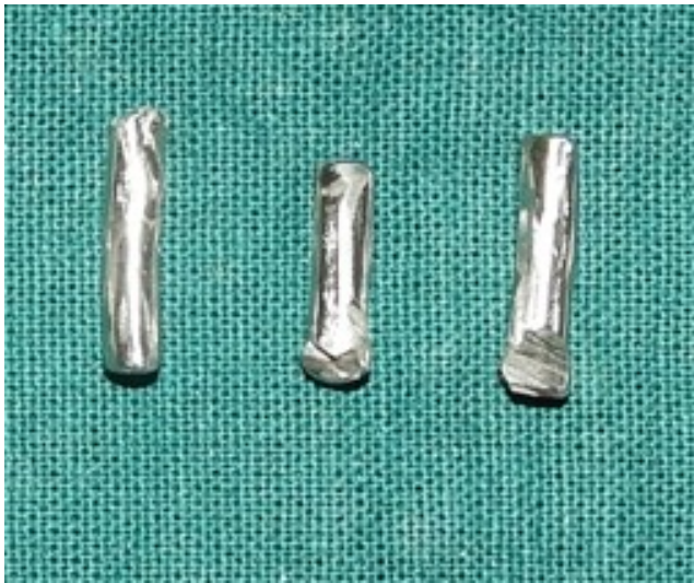
Fig. 2: Metal casted sprue of length 5mm.
