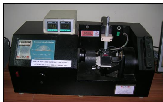
Fig. 2: Contact angle analyzer (Digidrop, Contact angle meter, GBX products, France)
