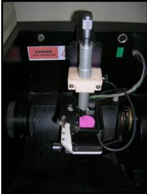
Fig. 3: Saturated solution of calcium sulphate dihydrate dispensed over the surface of the sample using calibrated microburette
