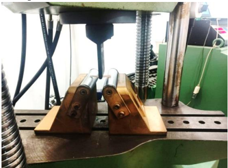
Figure 6: Specimen under 3 point bending test
