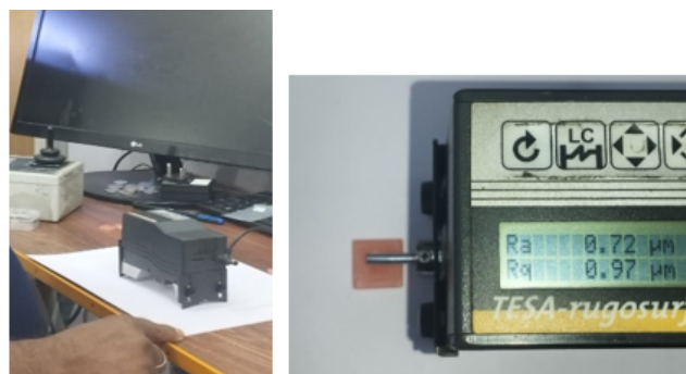
Figure 8: Testing of finished samples using portable surface roughness tester {TESA rugosurf10}
