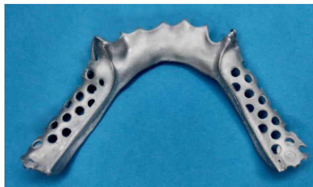
Figure 4: Cast partial denture framework fabricated using DMLS technology.
